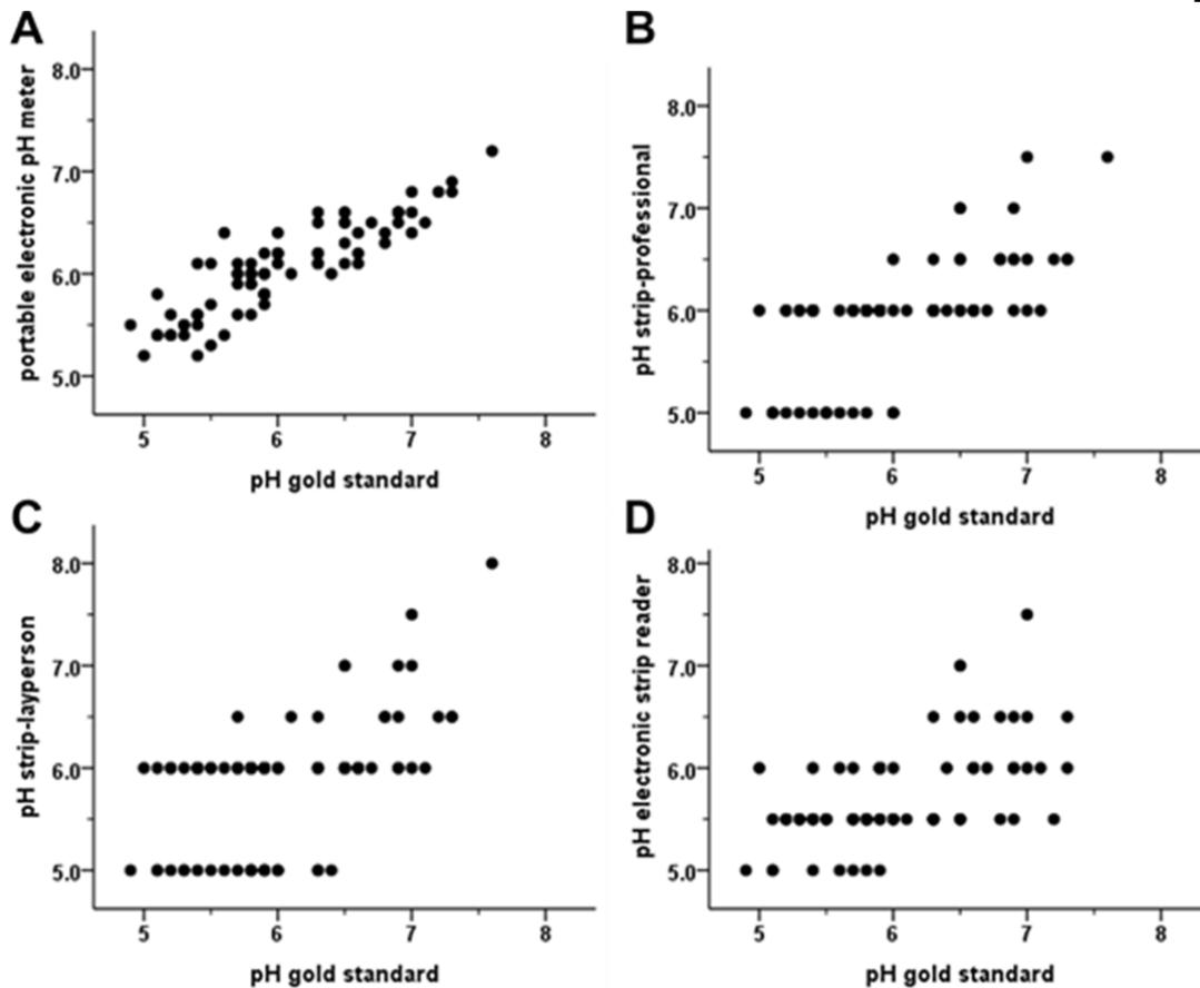
**Figure 1 : Correlation of gold standard versus other pH measurement methods**
